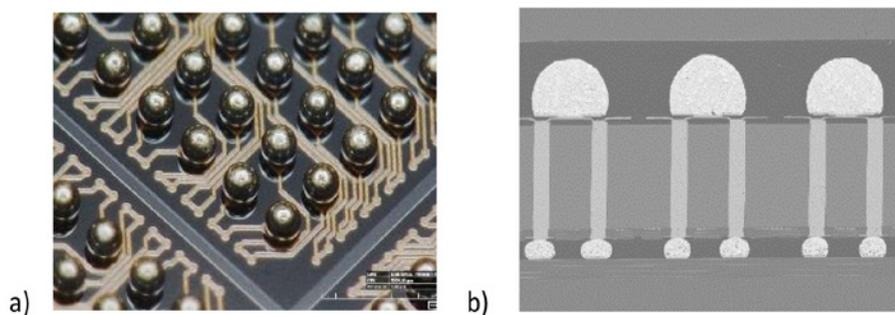
Figure 4: a) C4 bump + RDL for fan-in example; b) TSV insertion in active CMOS for 3DHI solution example.
