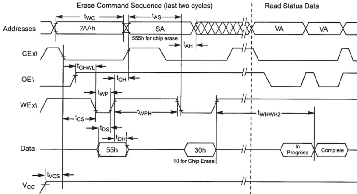
**NOTE:** SA = sector address (for Sector Erase), VA = Valid Address for reading status data (see "Write Operation Status").
