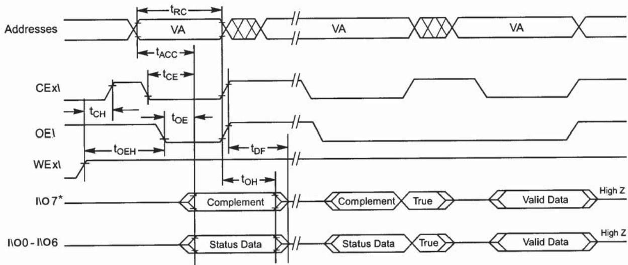
**NOTES:** VA = Valid address. Illustration shows first status cycle after command sequence, last status read cycle, and array data read cycle.
