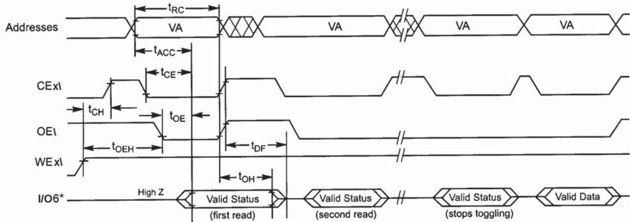
**NOTES:** VA = Valid address; not required for I/O6. Illustration shows first two status cycle after command sequence, last status read cycle, and array data read cycle.
