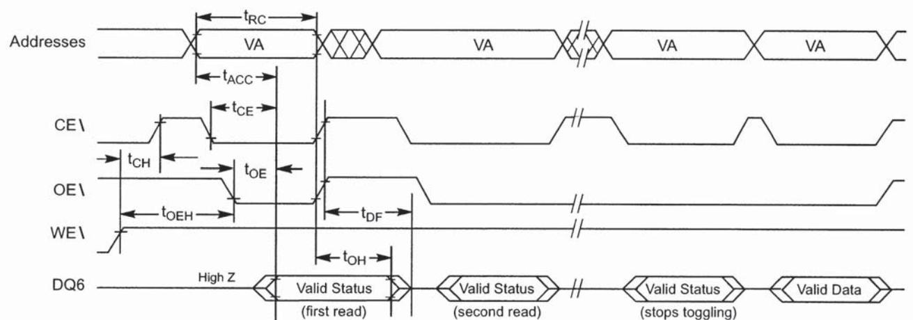
**NOTES:** VA = Valid address, not required for DQ6. Illustration shows first two status cycle after command sequence, last status read cycle, and array data read cycle.
