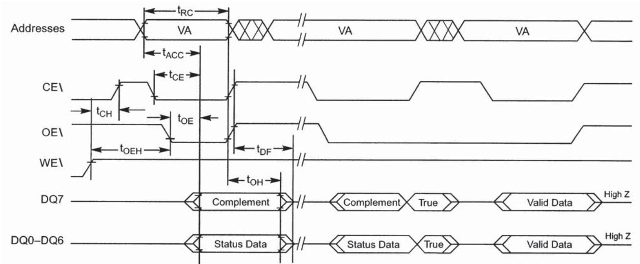
**NOTES:** VA = Valid address. Illustration shows first status cycle after command sequence, last status read cycle, and array data read cycle.
