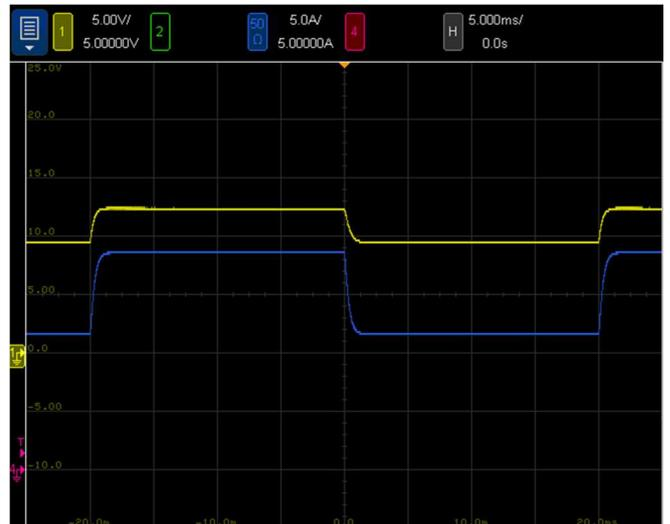
Fig. 9. Output current setpoint change with diode load (fifteen BYV32F in series). Output voltage is uncontrained. CH1: Output Voltage, CH3: Output Current
