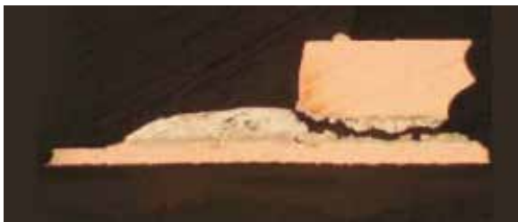
The Issue: Open Solder Joint
