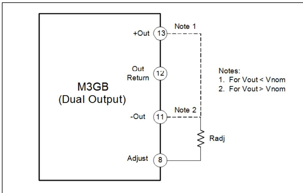
**Figure 4 Configuration for Adjusting Dual Output Voltage**
