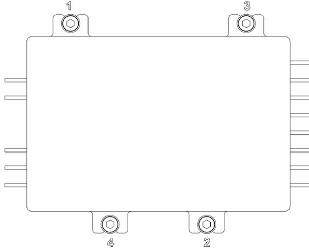
5. Tighten the screws with an appropriate torque driver. Torque the screws up to 6 in·lb in the sequence shown above
