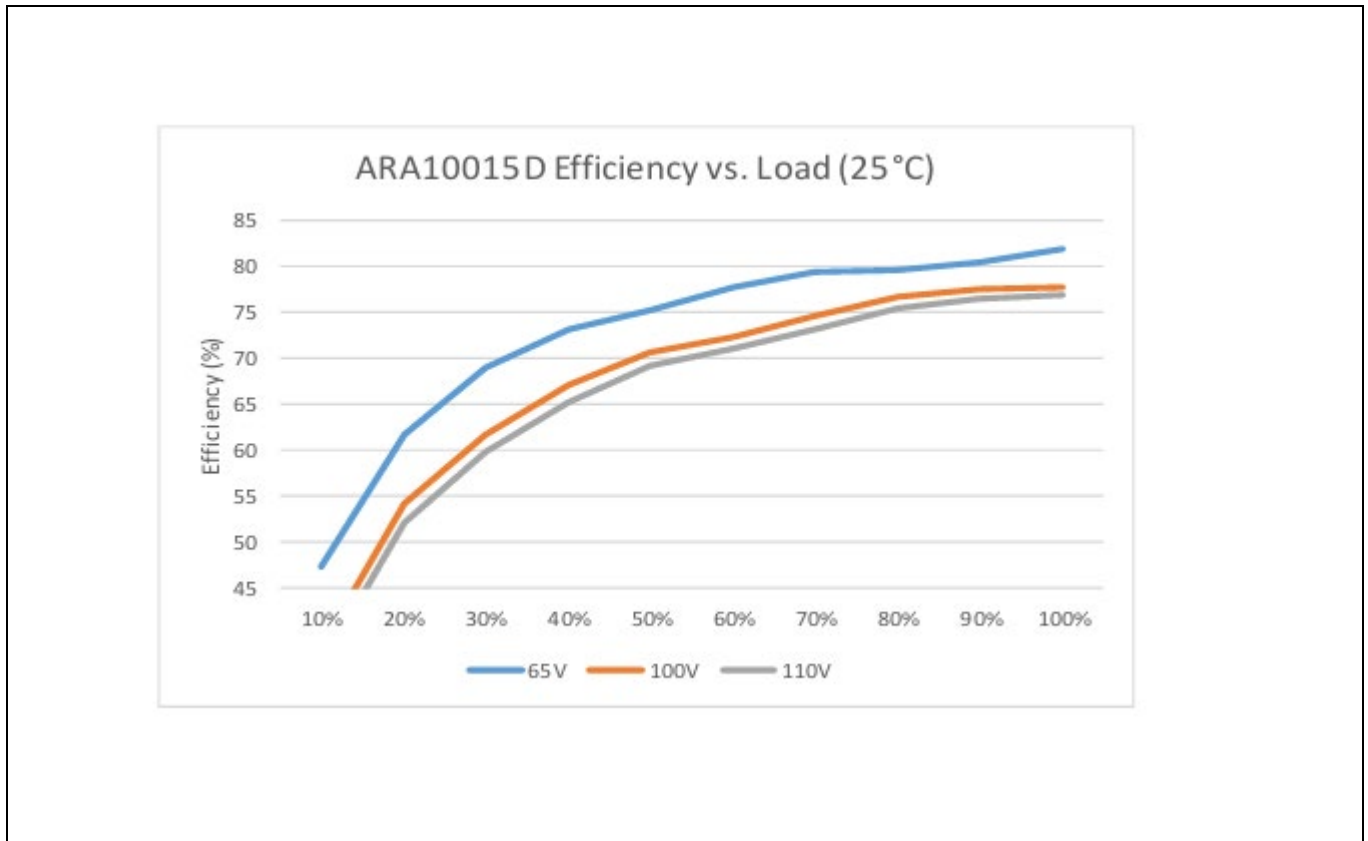
Figure 7 ARA10015D Efficiency vs. Load (25°C)
