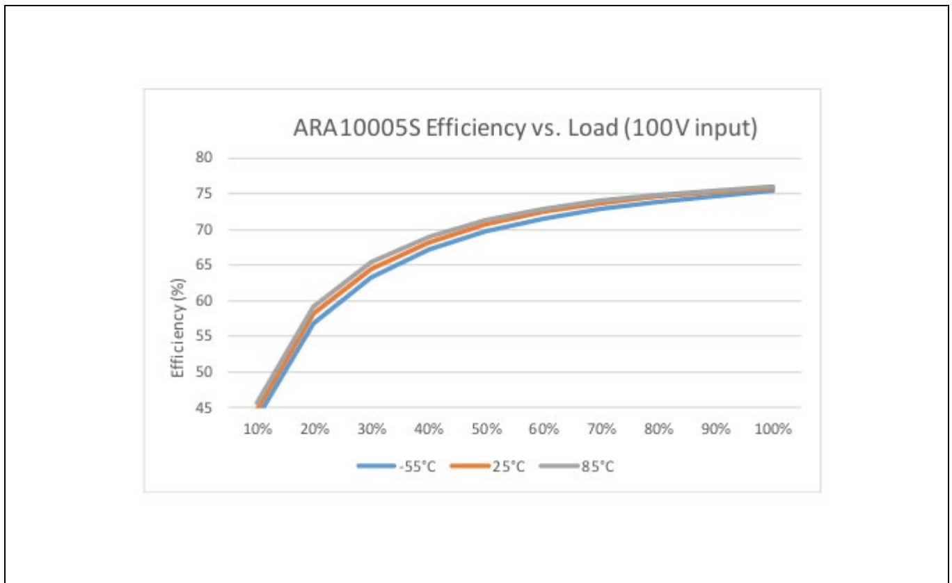
Figure 4 ARA10005S Efficiency vs. Load (100V input)
