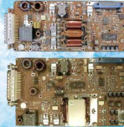
Micross EGB converters offer state of the art performance and is specifically designed for RF GaN SSPA applications. The EGB provides excellent efficiency and low CE, and can be tailored to the specific spacecraft bus and equipment requirements.
