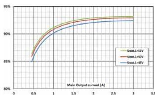
All 4 Outputs Loaded Equal Relative to Max Load
